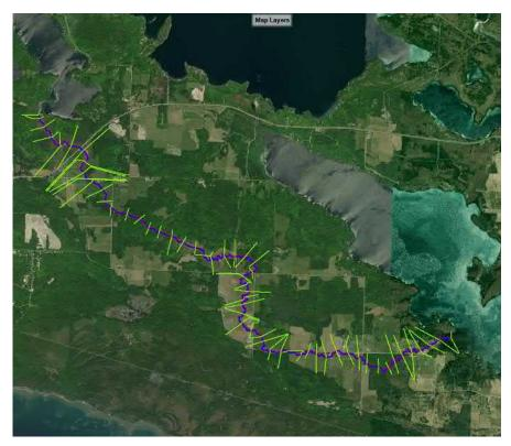
Figure 4-17: Pickerel Creek Model River and Cross-Section Layout
