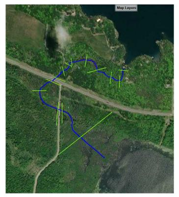
Figure 4-15: Harris Creek Model River and Cross-Section Layout
