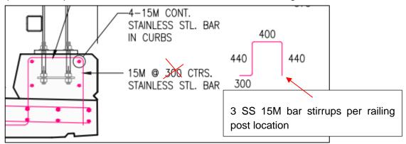
5. S4 Concrete Deck Plan indicates a stirrup 15M @ 300 ctrs typical both sides and shown on Section 1/S4. However, the dimension for this strip is not provided. Please review and advise.
